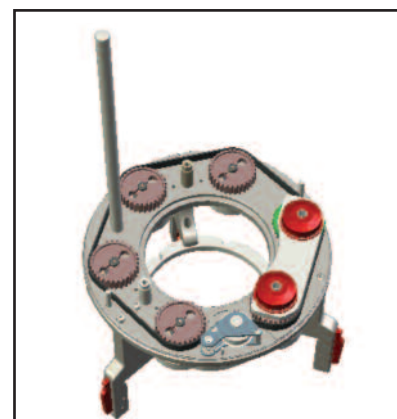
Cover removed showing drive belt and internal drive set-up
