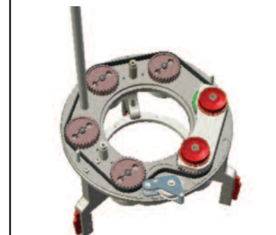
Tensioner in the release position to allow removal of the drive belt
