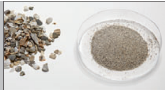
Stones before and after grinding with the Cross Beater Mill PULVERISETTE 16
