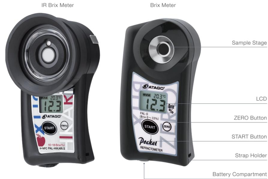
A combo set that includes PAL-HIKARI, a non-destructive IR Brix Meter that can measure the sugar content just by being pressed against the fruit, and a Brix meter that can measure the sugar content of squeezed fruit juice is now available. Special scales are available for each fruit. Choose the appropriate combo set.
