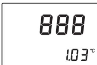
2. While continuing to hold the **ON/OFF** key, press the **ZERO** key. The temperature unit will change from °C to °F or vice versa.
