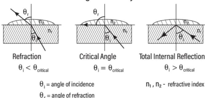
In the **MA882**, **MA883**, **MA884** and **MA885** refractometers, light from an LED passes through a prism in contact with the sample. An image sensor determines the critical angle at which the light is no longer refracted through the sample.
