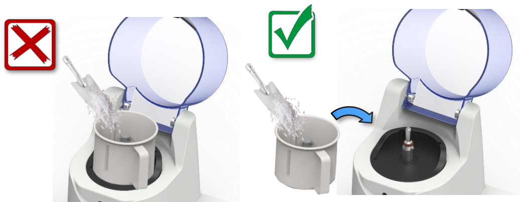
Fig. 3: Correct filling when grinding using dry ice and sample
